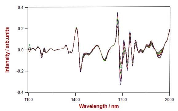
This Application Note describes a fast method for the simultaneous quantification of nicotine and glycerin in liquid mixtures used for electronic cigarettes. With visible near infrared spectroscopy (VIS-NIRS), results are available without sample preparation, thus making VIS-NIRS highly suited for fast quality control.
