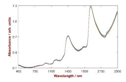
Fig. 2: Raw Vis-NIR spectra of 37 toothpaste samples over the full wavelength range.
