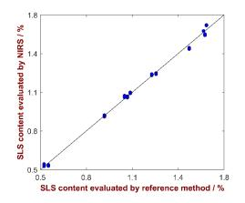
Fig. 4: Correlation plot of the SLS content predicted by NIRS versus the reference values. A high correlation is observable.
