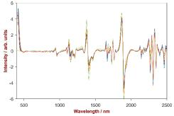
Fig. 4: 2- derivative and SNV pre-treatment of sample spectra.
