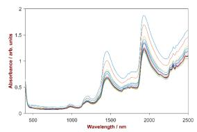
Fig. 3: Vis-NIR spectra of 12 sunscreen samples with differing SPF from 10 to 50.
