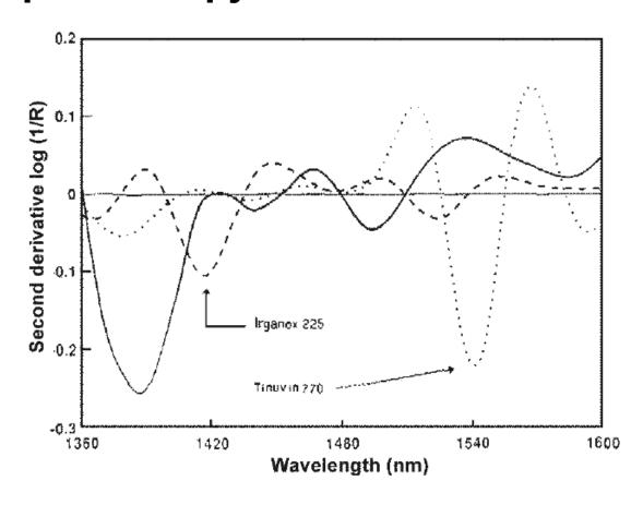
This Application note shows that NIR spectroscopy is an excellent tool for determining low levels of additives in finished polypropylene pellets. This is demonstrated by monitoring the UV stabilizer Tinuvin 770 and the antioxidant Irganox 225. Multiple linear least-squares regression (MLR) models compensate for pathlength variations and interferences in the polymer pellets.
