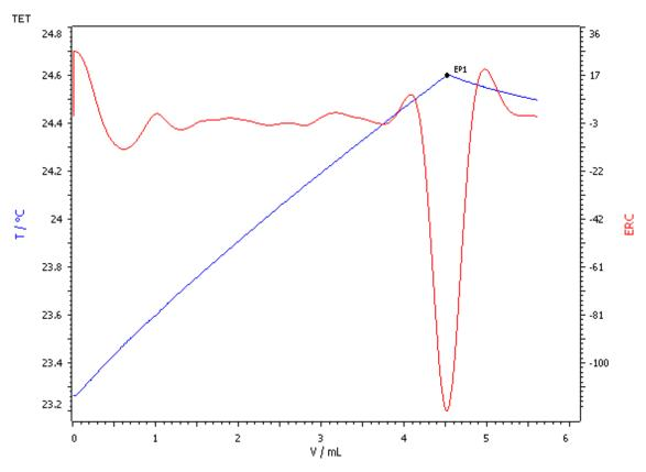
Hydrochloric and nitric acid can be determined in etching baths by thermometric titration. In a first titration the total acid content is determined by titration with sodium hydroxide. In a second titration the hydrochloric acid content is determined by titration with silver nitrate.
