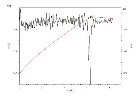
This Application Note describes a direct thermometric endpoint titration (TET) for the determination of concentrated potassium hydroxide solutions which had been used for the etching of substrates containing silicon.
