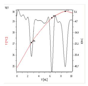
Thermometric titration plot of a mixture of  $H_3PO_4$ ,  $HNO_3$ , and  $CH_3COOH$  with 2 mol/L NaOH.
