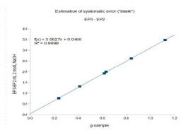
Blank determination EP3 - EP2 = 0.0466 mL
