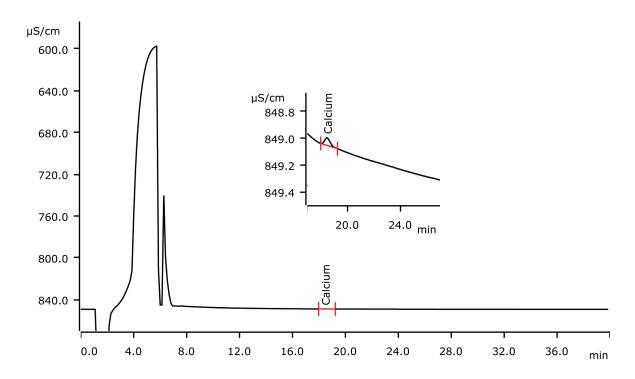
To refine bauxite to alumina, the bauxite ore is digested under pressure with a sodium hydroxide solution at a temperature between 150 and 200 °C. Trace analysis of calcium in the resulting Bayor Liquor requires dilution and pH adjustment. This is accomplished in a single step with 170 mmol/L citric acid. The citric acid sets the sample pH to approximately 4.5 and prevents aluminum precipitation. The separation is done on a Metrosep C 4 - 150/4.0 column with a citric acid eluent.
