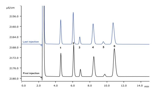
The stability of the Metrosep C 6 - 250/4.0 has been tested under lab conditions. For six consecutive days, two series of injections were done  $-9 \times$  tap water,  $3 \times$  check standard,  $6 \times$  tap water -; on the 7th day, the system was shut down. The instrument was running for over 10 weeks with a total of 2150 injections. The excellent data reproducibility underlines the very stable column performance.
