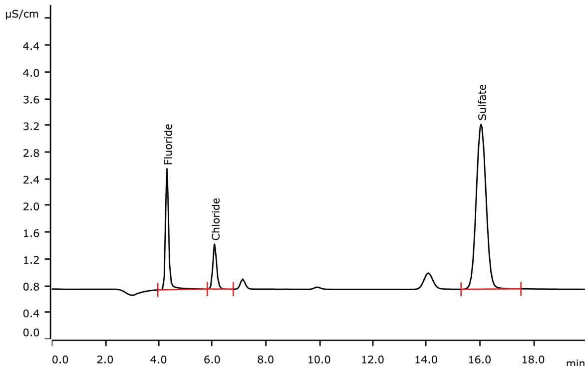
Clay is used for tile production. Quality control issues require the determination of its halogen and sulfur content. This is ideally done by Metrohm Combustion IC, where sulfur is detected as sulfate and the halogens as their corresponding halides. As clay often has high contents of alkali and alkaline earth metals that attack the pyrolysis tube, tungsten oxide is added before combustion.
