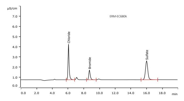
Combustion IC combines pyrohydrolytic sample combustion and absorption of the evolving combustion gases in an oxidizing aqueous solution that is then fed into an ion chromatograph for analysis of halides and sulfur (as sulfate). The combustion and analysis of certified reference materials (CRMs) proves the reliability of the Metrohm Combustion IC.
