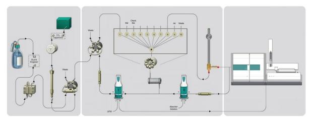
The transfer of samples and standards into the loop of the 920 Absorber Module is performed by the 5 mL Dosino using Metrohm intelligent Partial Loop Injection Technique (MiPT). The injection volumes are variable and range between 4 and 200  $\mu$ L. After Inline Matrix Elimination of excess  $H_2O_2$ , the sample is injected. No internal standard is required, as MagIC  $Net^{TM}$  considers all volumes that have been dosed into the combustion and absorption part.
