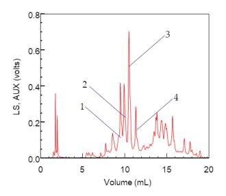
Figure 1. Reverse-phase chromatogram of gluten with the four peaks of interest identified.
