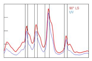
Figure 2. Selection of peak regions 1-4, showing light scattering signal at  $90^{\circ}$  (red) and UV absorbance signal (blue).
