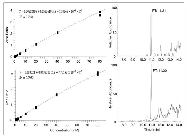
Figure 2. Left: Calibration curves of testosterone in fortified stripped plasma. Right: Corresponding XIC at the LLOQ level in plasma for testosterone (0.125 nM). Top and bottom: Data according to HR full-scan or targeted SIM acquisitions, respectively.
