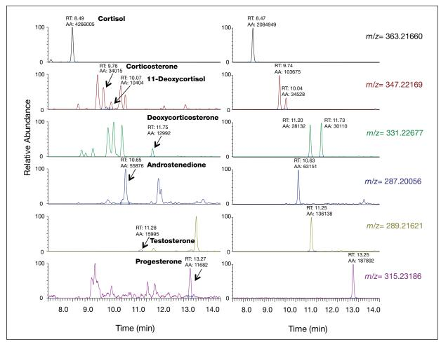
Figure 1. Example of XIC chromatograms extracted from HR full scan acquisition. Left: a male donor plasma sample. Right: a calibrator sample (stripped plasma fortified). Extracted *m/z* is listed on the right.
