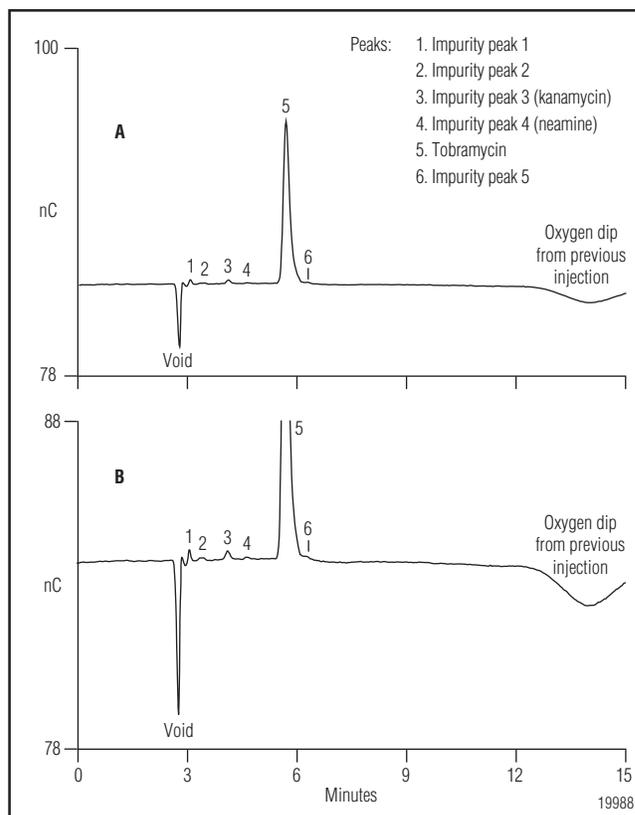
**Figure 3.** Determination of tobramycin ( $1.07\ \mu\text{M}$ , 20- $\mu\text{L}$  injection) using eluent generation (2 mM KOH) with 0.5 mL/min flow rate,  $30\text{ }^{\circ}\text{C}$  column temperature, and AAA-Direct waveform. Full view (A) and expanded view of baseline (B).
