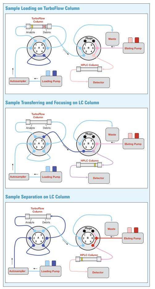
Figure 1: Transcend TLX dual-column configuration
