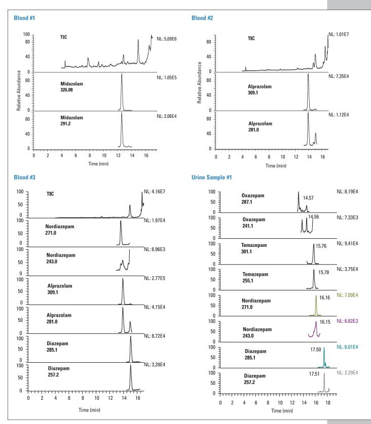
Figure 7: Chromatograms of benzodiazepines in human post-mortem blood and urine samples
