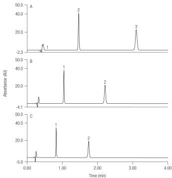
Figure 3. Representative chromatograms observed when increasing the method flow rate on an Accucore C8,  $100 \times 2.1$  mm,  $2.6 \ \mu m$  column.
