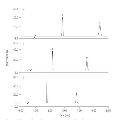
Figure 1. Separation of fenoprofen and gemfibrozil on three different columns A) Hypersil GOLD, 150 mm  $\times$  4.0 mm, 5  $\mu m$ , B) Accucore XL, C8 150  $\times$  4.6 mm, 4  $\mu m$ , C) Accucore C8, 100  $\times$  4.6 mm, 2.6  $\mu m$ .
