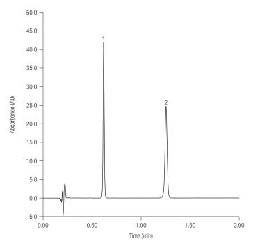
Figure 8. Overlay of 24 replicate injections of the standards mixture using the final developed method on an Accucore C8,  $100 \times 2.1$  mm,  $2.6 \mu m$  column,  $1.0 \mu m$ /min,  $45 \, ^{\circ}$ C.
