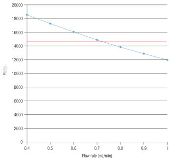
Figure 4. Plate count values when increasing the method flow rate on an Accucore C8,  $100 \times 2.1$  mm, 2.6  $\mu m$  column. The red line represents the 80% value of the plate count at 0.4 mL/min and the limit for USP equivalence.
