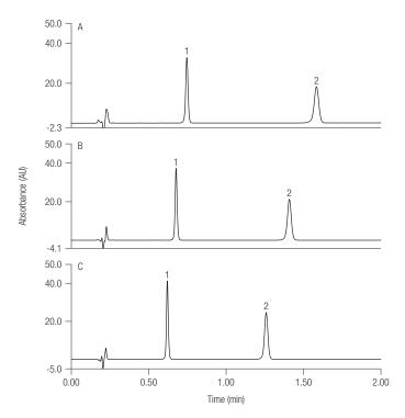
Figure 5. Chromatogram showing standards mixture analyzed on an Accucore C8, 50  $\times$  2.1 mm column at three different temperatures A) 25 °C, B) 35 °C, and C) 45 °C.
