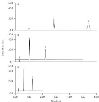
Figure 7. A comparison of the key stages of the method development. A) Original USP method, Hypersil GOLD, 150 mm  $\times$  4.6 mm, 5 µm column, 2 mL/min, 25 °C, B) Scaled USP method, Accucore C8, 100  $\times$  2.1 mm, 2.6 µm column, 0.7 mL/min, 25 °C, C) Beyond USP method, Accucore C8, 100  $\times$  2.1 mm, 2.6 µm column, 1.0 mL/min, 45 °C
