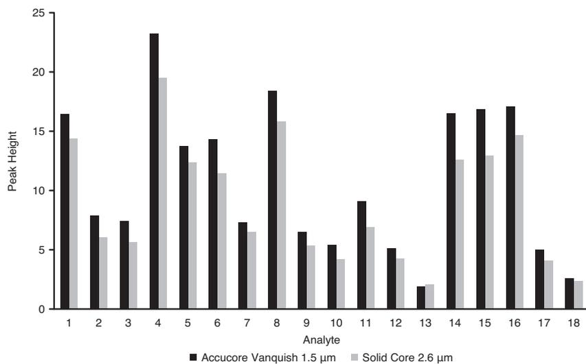
Figure 7: Comparison of peak height between the Accucore Vanquish UHPLC column and a 2.6  $\mu\text{m}$  solid core column
