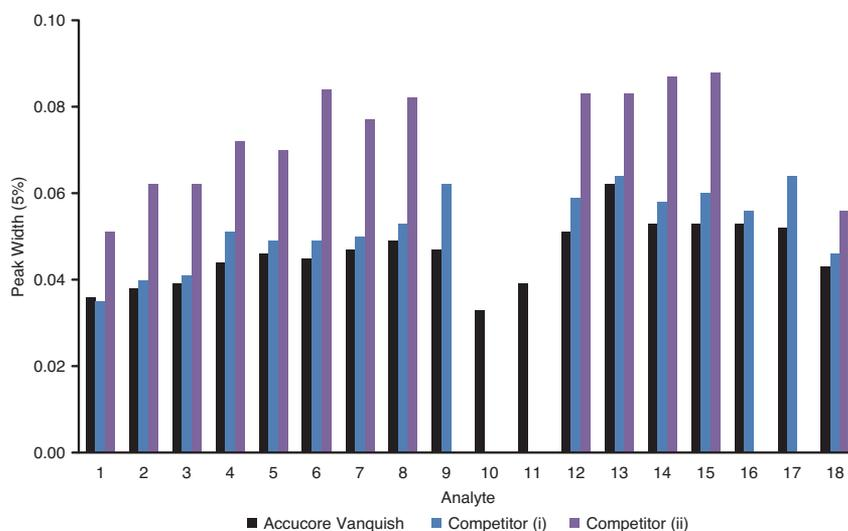
Figure 2: Comparison of peak widths for the Accucore Vanquish UHPLC column (black), competitor (i) (blue) and competitor (ii) (purple) columns. Peaks 10 and 11 coelute on competitor columns (i) and (ii).
