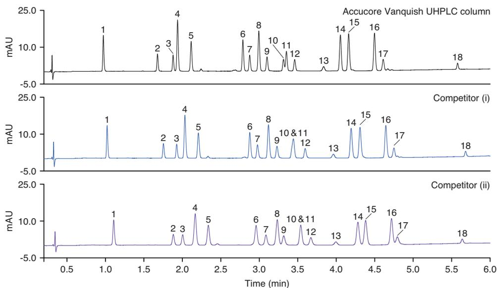
Figure 1: Chromatographic separation of eighteen herbicides on Accucore Vanquish UHPLC column (black), competitor (i) (blue) and competitor (ii) (purple) columns
