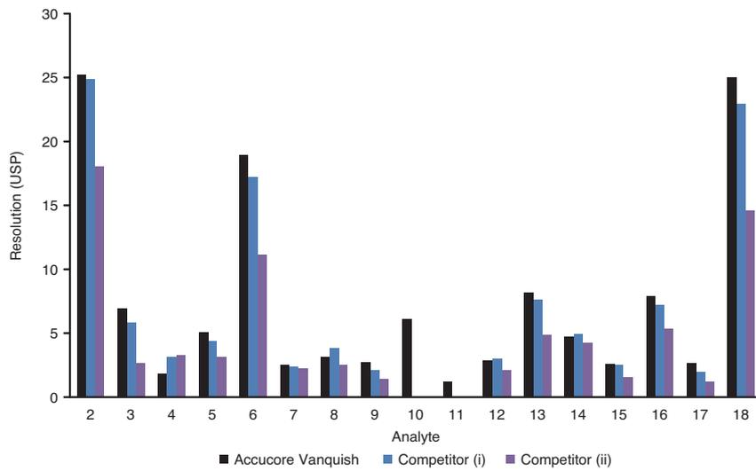
Figure 3: Comparison of resolution between the Accucore Vanquish UHPLC column (black), competitor (i) (blue) and competitor (ii) (purple) columns. Peaks 10 and 11 coelute on competitor columns (i) and (ii).
