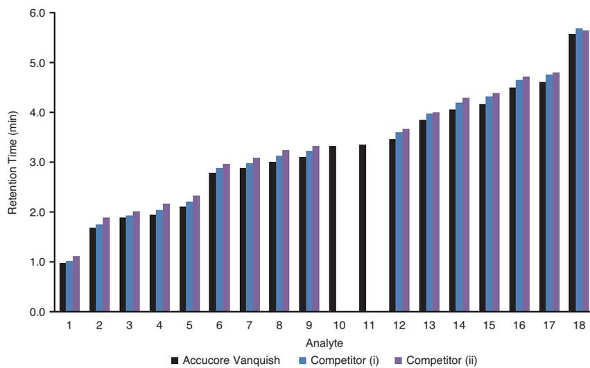
Figure 5: Comparison of retention times on the Accucore Vanquish UHPLC column (black), competitor (i) (blue) and competitor (ii) (purple) columns. Peaks 10 and 11 coelute on competitor columns (i) and (ii).
