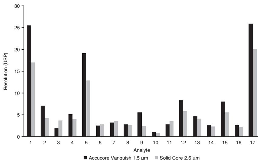
Figure 8: Comparison of resolution between the Accucore Vanquish UHPLC column and a 2.6 µm solid core column
