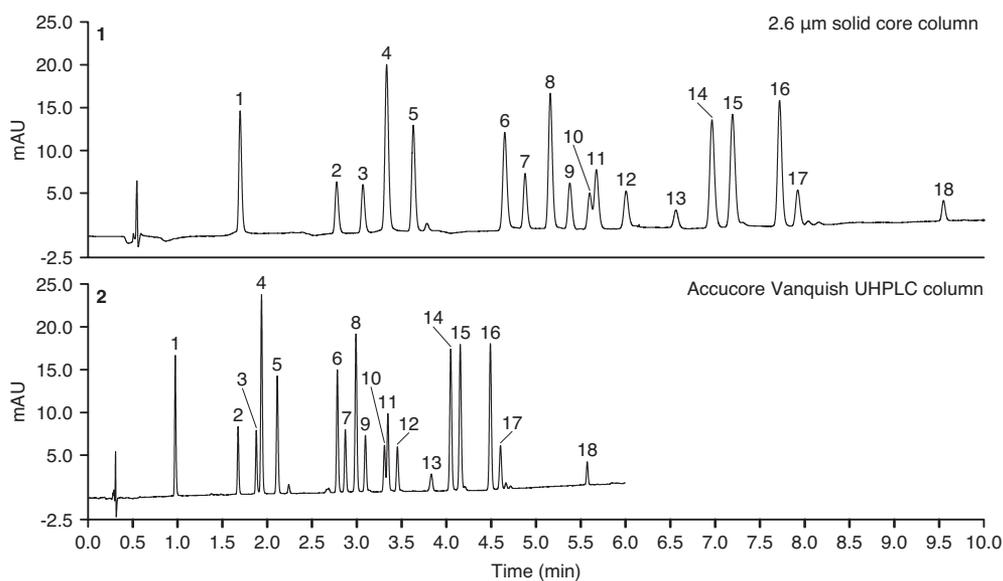
Figure 6: Chromatographic separation of 18 herbicides on a 2.6  $\mu\text{m}$  solid core column (top) and the Accucore Vanquish UHPLC column (bottom)
