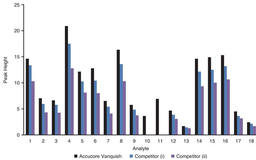
Figure 4: Comparison of peak height on the Accucore Vanquish UHPLC column (black), competitor (i) (blue) and competitor (ii) (purple) columns. Peaks 10 and 11 coelute on competitor columns (i) and (ii).
