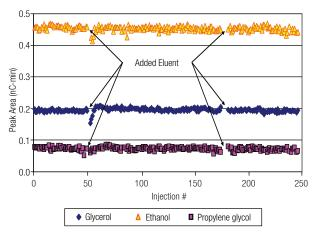
Figure 5. Peak area stability of 50 μM glycerol, propylene glycol, and ethanol spiked into a 300-fold dilution of the supernatant from heat quenched and centrifuged American Wheat *S. cerevisiae* incubated in Bacto YPD.
