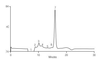
Figure 10. 40 µM glycerol and 400 µM ethanol spiked into a 400-fold dilution of German lager.
