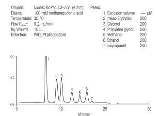
Figure 2. Separation of *meso*-erythritol, glycerol, propylene glycol, ethanol, methanol, and isopropanol.
