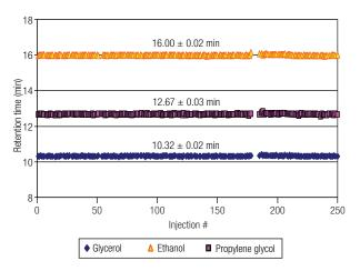
Figure 4. Retention time stability of 50  $\mu$ M glycerol, propylene glycol, and ethanol spiked into a 300-fold dilution of the supernatant from heat quenched and centrifuged American Wheat S. cerevisiae incubated in Bacto YPD.
