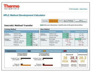
Figure 1: Isocratic method transfer calculator used in this application note to scale down the original USP chromatographic conditions [1]
