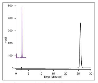
Figure 2: Chromatograms of 100  $\mu$ g/mL of zidovudine separated on a Syncronis C18 1.7  $\mu$ m, 50 x 2.1 mm column (top chromatogram), and on a Syncronis C18 5  $\mu$ m, 250 x 4.0 mm column (bottom chromatogram)
