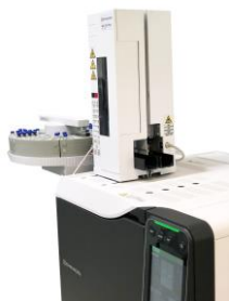
Figure 1: Dual AOC-20i/s Autosampler on Nexis GC-2030
