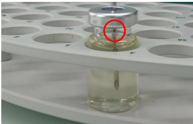
Figure 2: Sample vial filled up to the shoulder with immersed needle. The middle hole (red circle) is not immersed in the sample.
