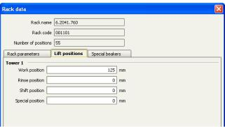
In order to configure the settings of the Liquid Handling Station, two external needle positions have to be defined for the tower of the Sample Processor in the window configuration. At the "external position 1" the needle should be in the inner compartment of the rinsing part which corresponds to an angle of approximately 106° and a work position of 125 mm. The exact angle depends on your installation. In this position, the needle is rinsed from the inand outside.
