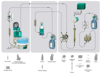
Prepare and degas an eluent suitable for the column you want to use (see column manual). For Metrosep A Supp 15 - 150/4.0 a solution of 5.0 mmol/L  $\rm Na_2CO_3$  / 0.3 mmol/L  $\rm NaOH$  is recommended.
