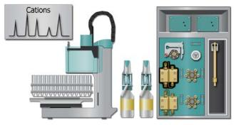
Now assign the following equipment: Assign the eluent to the IC pump (Pump 2) and define a reasonable start-up time, e.g. 2 minutes. In the analysis "Cation" link the corresponding pump (Pump 2); Data source (Conductivity Detector 2, Conductivity); injection valve (Injector 2) and column. Set the temperature of the column oven to 45°C.
