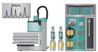
Now assign the following equipment: Assign the suppressor solution to the IC peristaltic pump and set the speed rate to 1, add your Rotor to the MSM and activate the automatic stepping all 10 minutes, assign the eluent to the anion IC pump (Pump 1) and define reasonable start-up times e.g. 2 minutes. Set the temperature of the column oven to 45°C.
