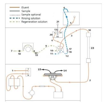
Make sure that all outlet capillaries are put into the waste collector.
