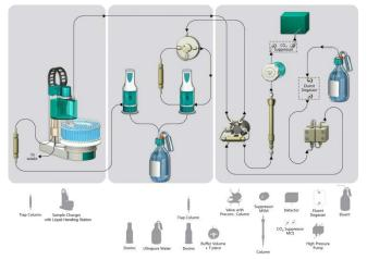
Prepare and degas an eluent suitable for the column you want to use (see column manual). For Metrosep A Supp 15/4.0 a solution of 5.0 mM  $Na_2CO_3$  / 0.3 mM NaOH is adequate.
