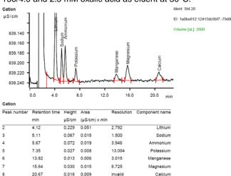
In the application work CH6-0911-112007, exemplary measurements were performed with the ProfIC Vario 5 setup. A Metrosep C  $_3$  -150 column was used. The calibration was performed within the concentration range of 0.5  $_-$  10 ppb, and a linear curve type was used for evaluation. Correlation coefficients and standard deviations are listed in the following table. The calibration curve for lithium is shown as an example.
