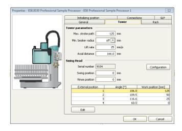
In the sub-ppb analysis all contaminations have to be avoided. To have a possible source of contamination under control, it is important to move the needle of the Sample Processor to a defined position after initialization. For this, please add an initial position which is equal to the external position 1 in your configuration:
