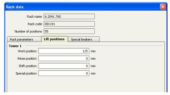
For using the Liquid Handling Station, it is necessary to define external positions for the needle. This is done in the configuration of the Sample Processor in the subtab "Tower". Please define the external positions 1 and 2 according to the picture below. Attention: The angles are only approximate values, for fine tuning, please use the manual control to find the correct values for this system and adjust them then in the configuration.
