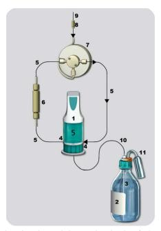
The Dosino is plugged in at the back of the Sample Processor. The method ProfIC Vario 5 Cation uses the MSB1 port of the IC for the Dosino.
