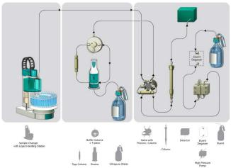
Prepare and degas an eluent suitable for the column you want to use (see column manual). For Metrosep C 4-150/4.0 a solution of 1.7 mmol/L HNO $_3$  / 0.7 mmol/L dipicolinic acid (DPA, 2,6-Pyridinedicarboxylic acid) is adequate.
