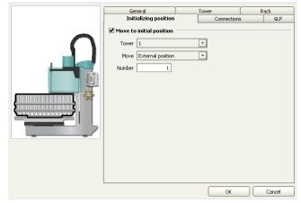
In the configuration of the solution LH Dosino, define the settings of the Dosing Unit. In the here present setup, an increased backpressure due to many capillary connections, Trap column and preconcentration column can be observed. For this reason it is important to define a maximum dosing rate for the Dosino. Also adjust length and diameter of your capillaries connected to the dosing unit. This is important to ensure complete rinsing of all connections when executing the prepare command.
