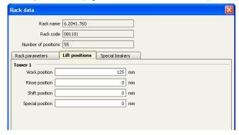
For using the Liquid Handling Station, it is necessary to define external positions for the needle. This is done in the configuration of the Sample Processor in the subtab "Tower". Please define the external positions 1, 2 and 3 according to the picture below. Attention: The angles are only approximate values, for fine tuning, please use the
