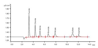
The calibration was performed with one standard containing standard anions of 20 ppm each. Within the concentration range of 0.2 - 10 ppm, a quadratic curve type was used for evaluation.
