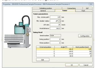
For the Dosino, the exact lengths and diameters of the tubings used need to be added for it to work properly. This can be done in the configuration as follows:
