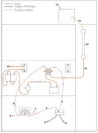
The sample injection is at position 1 of the valve. A counter current flow of the sample with regard to the eluent flow is recommended, in order to minimize diffusion and carry over. Make sure that all outlet capillaries are put into the waste collector.
