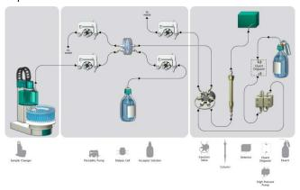
Prepare and degas an eluent suitable for the column you want to use (see column manual). For Metrosep C 4 - 150/4.0 a solution of 1.7 mmol/L HNO<sub>3</sub> / 0.7 mmol/L dipicolinic acid (DPA, 2,6-Pyridinedicarboxylic acid) is adequate.
