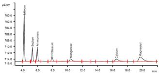
For the calibration, the average peak areas of 3 injections were evaluated. Within the concentration range of 1-20 mg/L, a linear curve type was used for evaluation. Correlation coefficients and standard deviations are listed in the following table. The calibration curve for lithium is shown as an example.
