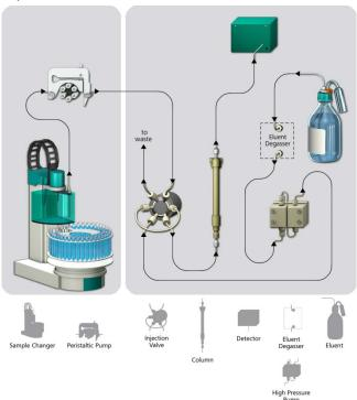
Prepare and degas an eluent suitable for the column you want to use (see column manual). For Metrosep C 4 - 150/4.0 a solution of 1.7 mmol/L HNO<sub>3</sub> / 0.7 mmol/L dipicolinic acid (DPA, 2,6-Pyridinedicarboxylic acid) is adequate.
