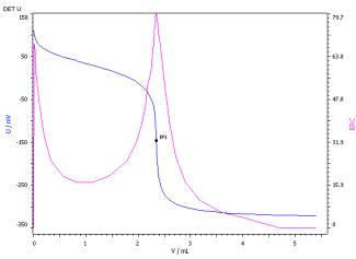
Fig. 1: Determination of the acid value (blue = titration curve, pink = ERC)
