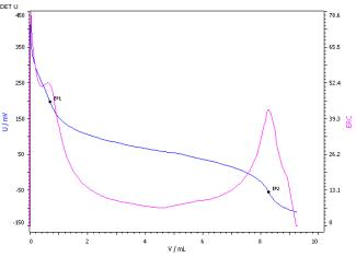
Fig. 2: Determination of the hydroxyl value (blue = titration curve, pink = ERC)
