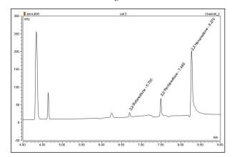
Figure 3. Calibration point chromatogram at 0.1 mg/L.
