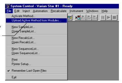
To upload the Method from the 3800 GC to System Control, select "Upload Active Method from Modules..." from the File menu.
