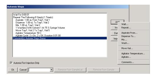
The Add and Insert buttons bring up a popup menu (above, right) showing the different commands that can be added. Based on the command selected, a dialog box is displayed to select its parameters.
