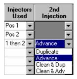
If "Advance" is selected, upon finishing the 1<sup>st</sup> injection the 8400/8410 will immediately move to the next vial position and withdraw sample from the vial and perform the 2<sup>nd</sup> injection. If "Clean & Adv" is selected, upon finishing the 1<sup>st</sup> injection the 8400/8410 will advance to the next vial position and then clean the syringe with wash solvent before proceeding with the 2<sup>nd</sup> injection.
