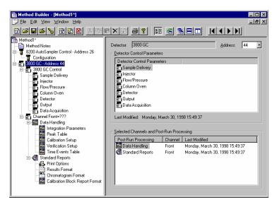
The 3800 Method section contains seven Method windows: Sample Delivery, Injector, Flow/Pressure, Column Oven, Detector, Output, and Detector Information. These windows contain all parameters that control the operation of the 3800 GC during a chromatographic run.
