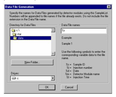
The right side of this dialog box allows you to create a filename "specification". You can combine text entry with the "%" variable symbols shown to specify filenames that contain sample injection specific information. An example of the filename is dynamically updated as you type in the filename specification. This makes it easy to see how a Data File created with this filename specifications would appear.
