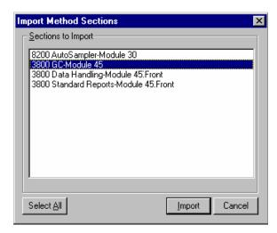
When the desired sections have been highlighted, click on the Import button to import them into the Method being edited. If the Method already has sections with the same module address and channel ID, you will be prompted to reassign a new module address and channel number to the imported section or overwrite the existing section in the current method.
