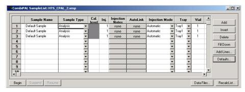
The Standard SampleList Columns are: Sample Name, Sample Type, Cal Level, Inj., Injection Notes, Autolink, Amount Std...,Unid. Peak Factor, Multiplier, Divisor, Internal Standard.
