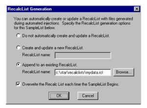
If you choose to create a new RecalcList, this automatically generated RecalcList will not overwrite an existing RecalcList unless you also specify "Overwrite the Recalc List each time the SampleList begins". If a RecalcList with the same filename exists, the newly created RecalcList will have number appended to its filename to make it unique and to prevent the older RecalcList from being overwritten.
