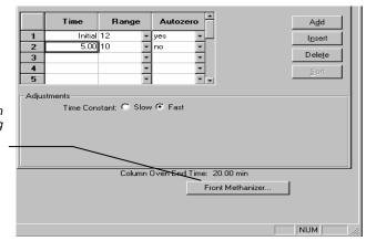
Program the Methanizer in the position corresponding to the tab in the Detector window by clicking on the Methanizer button.
