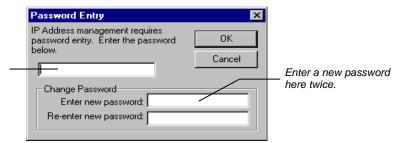
The initial password is blank (no password). To set your password initially, enter the desired password in the *Enter new password* and *Re-enter new password* fields. Subsequent entry into the BOOTP Server will require this password.
