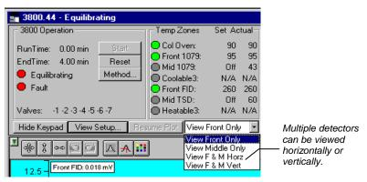
The component status display can be changed to view detailed status of each component in the GC.
