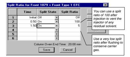
The first row of the spreadsheet contains the Initial Split State and Split Ratio for the 1079 injector. The 1079 will equilibrate to this setting when the method is activated, and will be restored to this setting when each chromatographic run is completed.
