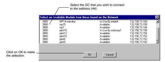
Repeat this procedure for up to four GCs (addresses 44 through 47) controlled by the Workstation.
