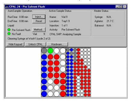
The left side of the window shows the Combi PAL Operation parameters: RunTime, EndTime, Injection Mode, Method State, Fault State, and current Vial location. The Inject, and Reset pushbuttons control the Combi PAL's immediate operation. The Method pushbutton opens Method Builder for editing of the active Combi PAL method.
