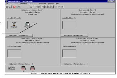
Double-click in this area or select the instrument from the Instrument menu to view the 3800 GC Status and Control window.
