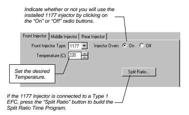
Note: You must have already configured the Type 1 EFC in the corresponding position in the Flow/Pressure Section before you can program the split ratio. Specifically, to build a 1177 Split Ratio Program, a Front 1177 must have a corresponding Front Type 1 EFC, a Middle 1177 must have a corresponding Middle Type 1 EFC, and a Rear 1177 must have a corresponding Rear Type 1 EFC.
