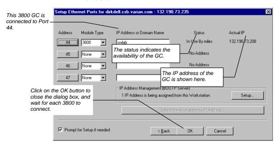
When each 3800 connects to System Control, it will be represented by an icon at the bottom of the Configuration Window. The icon will have a label reading 3800.44, through 3800.47 and will include the Host Name of the GC appended to the label. The numbers 44 - 47 are System Control communication addresses that correspond to the Ethernet port connected to the device.
