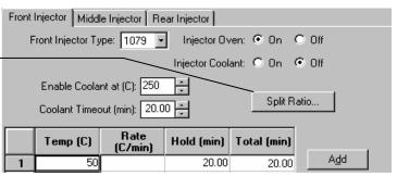
Note: You must have already configured the Type 1 EFC in the corresponding position in the Flow/Pressure Section before you can program the split ratio. Specifically, to build a 1079 Split Ratio Program, a Front 1079 must have a corresponding Front Type 1 EFC, a Middle 1079 must have a corresponding Middle Type 1 EFC, and a Rear 1079 must have a corresponding Rear Type 1 EFC.
