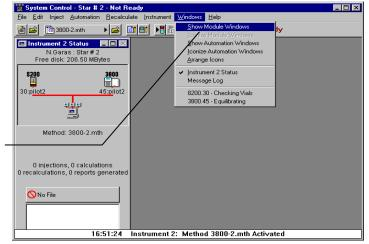
If the Status and Control Windows for the modules configured in the instrument are not currently displayed, you can select Show Module Windows from the Windows menu.
