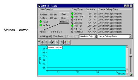
When you click on this button Method Builder is opened with active Method loaded and the corresponding Instrument Module selected. You can then edit that section or any other section of the Method as described previously.
