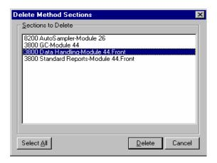
When the desired sections have been highlighted, click on the Delete button to delete them from the Method being edited. You will be prompted to confirm that you want to delete each section before it is deleted.
