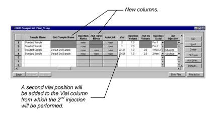
The "2<sup>nd</sup> Sample Name" column allows you to enter a unique sample name for the 2<sup>nd</sup> injection. You can also enter notes unique to the 2<sup>nd</sup> injection, and you can choose a different volume for the 2<sup>nd</sup> injection.
