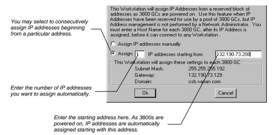
When the Assign # IP addresses starting from: #.#.# radio button is selected, the bottom portion of the dialog changes.
