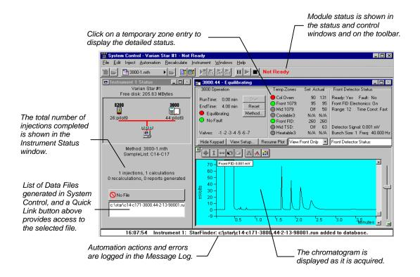
When you double-click on the status bar at the bottom of the instrument window, the entire Message Log window is displayed.
