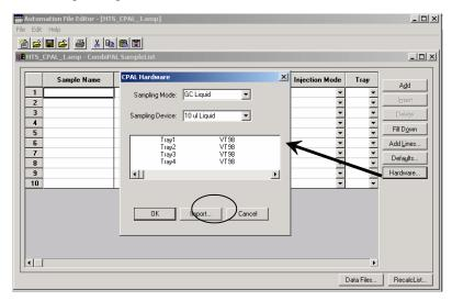
Because of the complexity of the CPAL Tray configurations, the sample list needs to be aware of all the hardware items, in particular the tray info and use this information to validate the sample location info. When the SampleList is edited in System Control (on-line), this information is automatically added to the SampleList.
