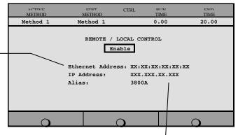
Use the Ethernet address shown here when setting up the BOOTP Server.
