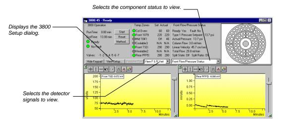
The detector signals viewed in the real time chromatogram display can be selected.
