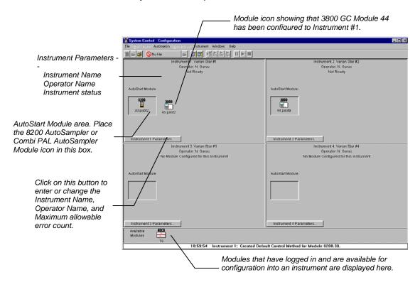
If the 3800 is to be operated with an 8400 AutoSampler or with the 8410 AutoInjector, the 3800 GC must be placed in the AutoStart Module.
