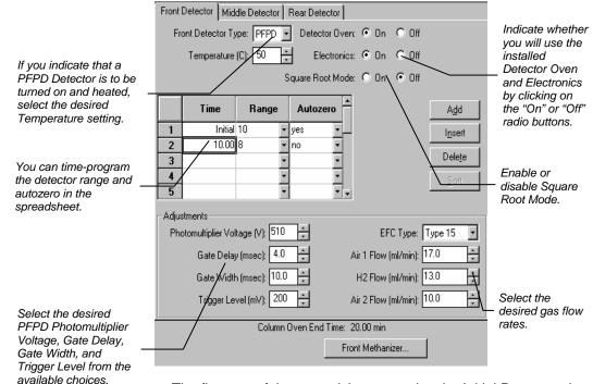
The first row of the spreadsheet contains the Initial Range and Autozero for the PFPD Detector. The PFPD will switch to this setting when the method is activated, and will be restored to this setting when each chromatographic run is completed.
