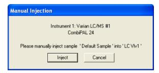
In GC mode, there is no Inject button in the Manual Injection dialog since the inject signal is triggered by the Automatic Start Switch that is part of the GC Injector.
