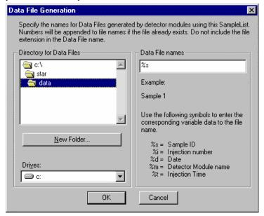
The right side of this dialog box allows you to create a filename "specification". You can combine text entry with the "%" variable symbols shown to specify filenames that contain sample injection specific information. An example of the filename is dynamically updated as you type in the filename specification. This makes it easy to see how a Data File created with this filename specification would appear.
