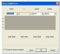
Now press the **OK** button to close the Dialog Box. The CPAL module address in System Control is derived from the serial slot number, as shown in the following table:
