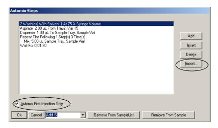
When you have finished creating an Automix routine you will need to give it a name by typing in the text box at the bottom of the Automix Steps screen. After pressing **OK**, this Automix routine will be added to the sample line and saved to the SampleList. Additional Automix routines can be saved to the same SampleList.
