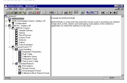
The first item in the Method is the Method Notes section. Method Notes is a free form text field where information about the Method or the application can be entered. Method Notes are displayed in the File Open dialog boxes used whenever you select a Method.
