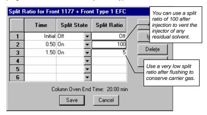
The first row of the spreadsheet contains the Initial Split State and Split Ratio for the 1177 injector. The 1177 will equilibrate to this setting when the method is activated, and will be restored to this setting when each chromatographic run is completed.
