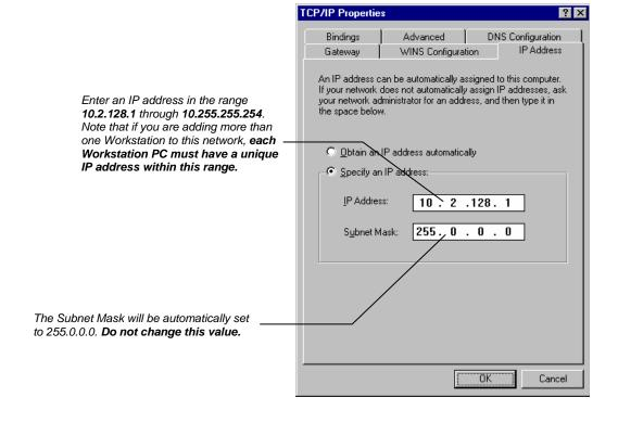
Ensure that no entries have been made in your Gateway, and that Domain Name Server (DNS) and WINS Configuration have been disabled. These entries are not used in an isolated network and may cause problems if they are present. Delete any settings that may have been entered from a previous configuration.
