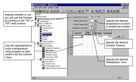
The first row of the spreadsheet contains the Initial temperature and hold time for the Column Oven. The Column Oven will equilibrate to this setting, and stabilize for the specified Stabilization Time, when the method is activated, and will be restored to this setting when each chromatographic run is completed.
