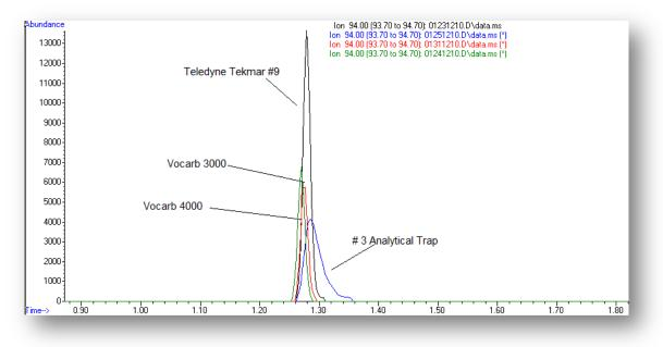
Figure 1: EICP of m/z 94 of Bromomethane for all four analytical traps evaluated at 10ppb.
