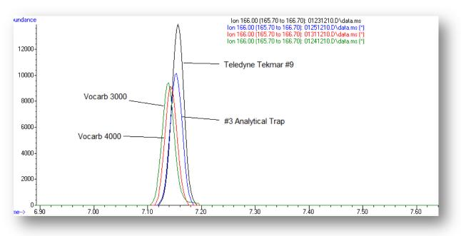
Figure 2: EICP of m/z 166 for Tetrachloroethylene for all four analytical traps evaluated at 10ppb.
