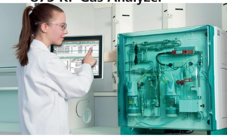
Straightforward determination of water content in liquefied and permanent gases
