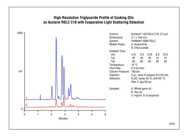
When comparing oils of similar properties, or trying to get a detailed profile of an oil, a high-resolution analysis is needed. The Acclaim 120 RSLC C18 2.2  $\mu$ m 2.1  $\times$  100 mm column provides excellent efficiency without a speed penalty. Selectivity is improved by using an acetonitrile/ethyl acetate gradient at sub-ambient temperature.
