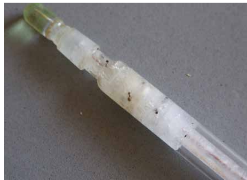
Figure 6: Electrode with completely crystallized reference electrolyte.
