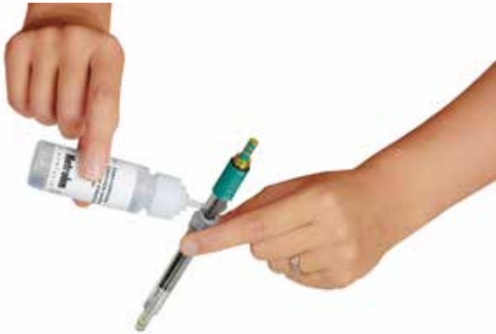
Figure 9: Shows an Unitrode which is refilled with electrolyte.
