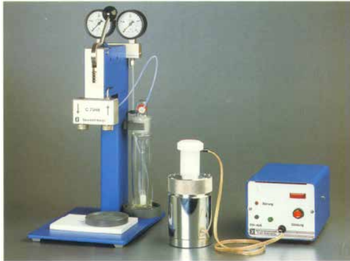
Figure 2: ADD digestion system (IKA)
