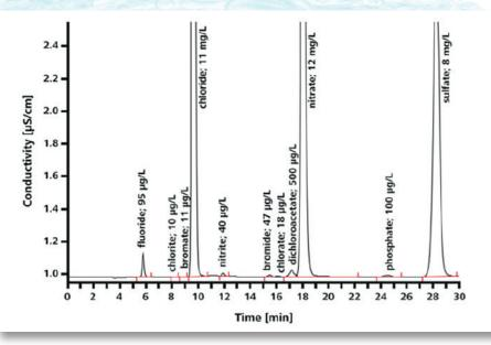
Metrosep A Supp 7 - 250 / 4.0: 3.6 mmol/L sodium carbonates, column temperature 45 °C, Sample volume 50 µL, flow 0.7 mL/min, Inline ultrafiltration, sequential suppression, conductivity detector
