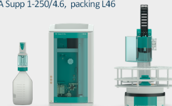
Fig 5. Ion Chromatography Instrument used for Fluoride Assay in OTC Products
