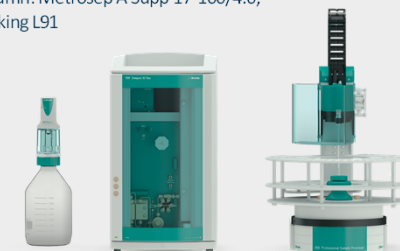
Fig 4. Ion Chromatography Instrument Used for Iodide Assay
