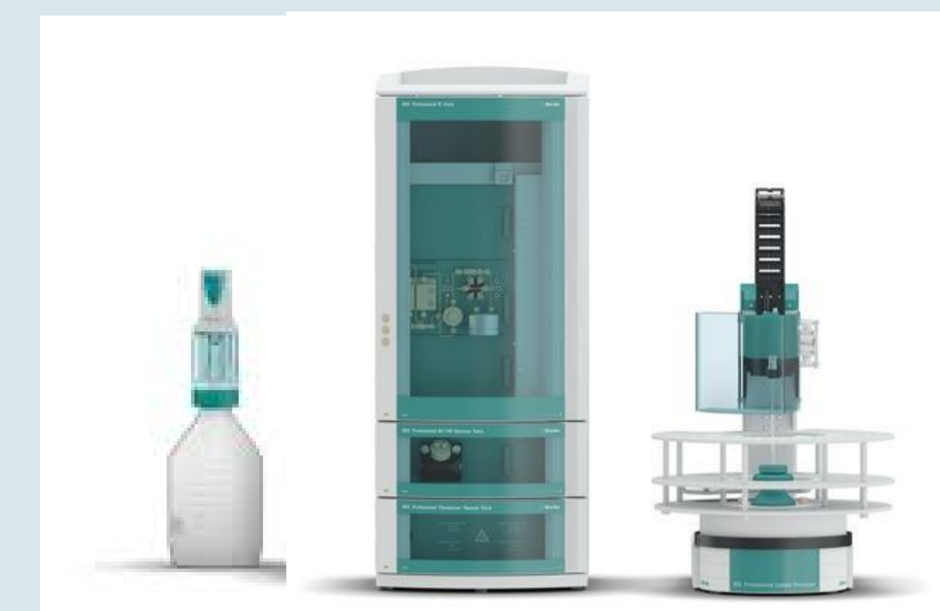
Fig 5: Ion Chromatography instrument used for OTC assay
