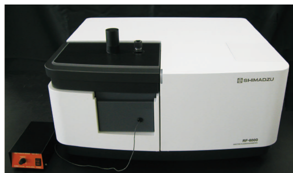
Fig. 1 RF-6000 Spectrofluorophotometer Coumarin (Diesel Oil Marker) Identification System
