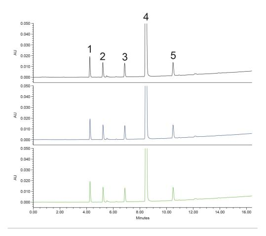
Figure 1. Stacked plot of chromatograms for three replicate injections of rivaroxaban and impurities analyzed using a 5–95% ethanol gradient on an XSelect Premier HSS T3 4.6 x 100 mm 3.5 µm Column. 1) Related Compound B, 2) Related Compound D, 3) Related Compound G, 4) Rivaroxaban, 5) Related Compound J. UV Detection at 250 nm.
