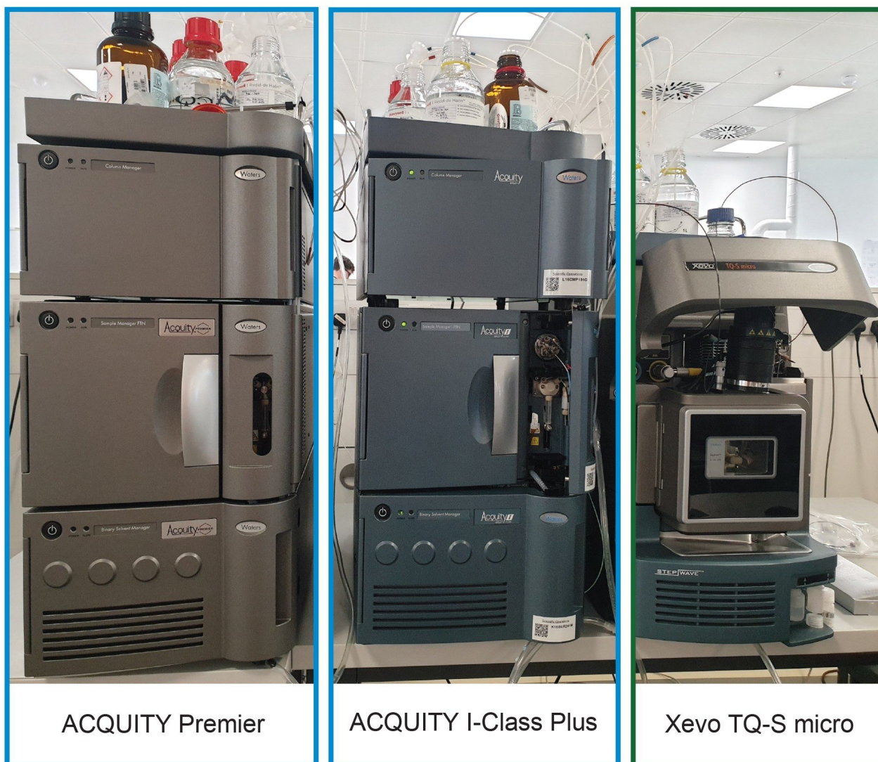
Figure 1. The configuration used in this work (from left to right: ACQUITY Premier, ACQUITY I-Class, and Xevo TQ-S micro).
