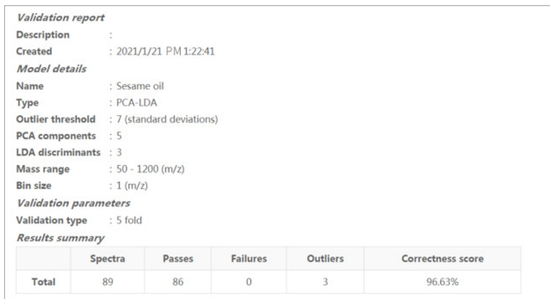
Figure 3. Cross-validation results of the model of edible oils adulteration based on RADIAN ASAP data.
