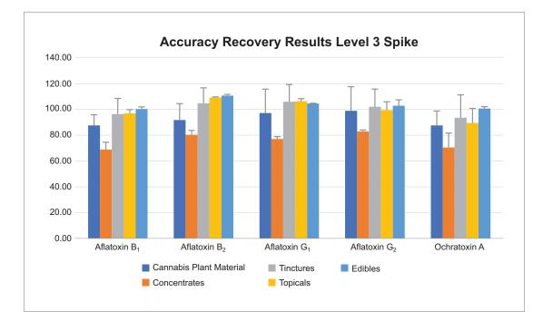
Figure 6. Accuracy Level 3: 12 ppb each individual Aflatoxin and 36 ppb Ochratoxin A for type B (cannabis plant material, topicals, tinctures, and edible) samples and 20 ppb each individual Aflatoxin and 60 ppb for Ochratoxin A for type A (concentrate) samples.
