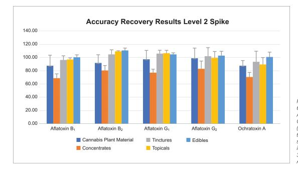
Figure 5. Accuracy Level 2: 6 ppb each individual Aflatoxin and 18 ppb Ochratoxin A for type B (cannabis plant material, topicals, tinctures, and edible) samples and 10 ppb each individual Aflatoxin and 30 ppb Ochratoxin A for type A (concentrate) samples.
