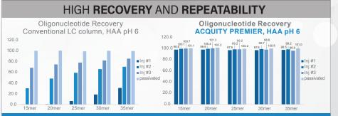
Injection of 2 µL of standard diluted in water, 10 pmol of each oligonucleotide injected on column.
