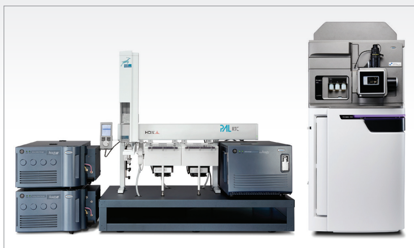
Figure 1. HDX MS workflow solution and the SYNAPT XS High Resolution Mass Spectrometer.
