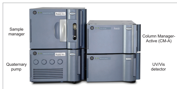
Figure 1. The ACQUITY Arc Bio System. The system is configured with a CM-A column compartment module that houses the valves for column selection between two columns. The quaternary pump enables the use of Auto•Blend Plus, which adjusts mobile phase pH and salt composition through the use of concentrated stock solutions.
