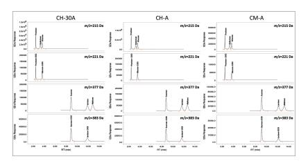
Figure 2. Chromatograms of sugar standards acquired on an ACQUITY Arc System with CH-30A, CH-A, and CM-A column compartments. The <sup>13</sup>C stable isotope labeled sugars were used as internal standards.
