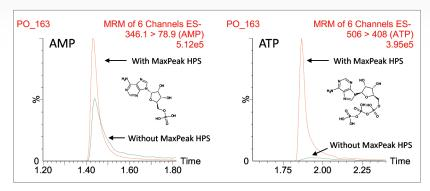
Figure 1. Separation of AMP (left) and ATP (right) on the Atlantis BEH C<sub>18</sub> AX sorbent with MaxPeak HPS column hardware (red line) and standard column hardware (green line).
