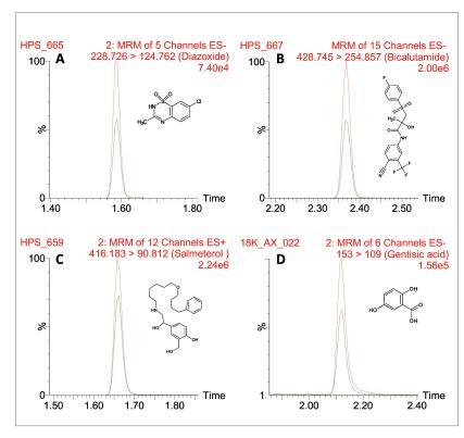
Figure 2. Peak area recovery of diazoxide (A), bicalutamide (B), salmeterol (C), and gentisic acid (D) on the Atlantis BEH  $C_{18}$  AX sorbent with MaxPeak HPS column hardware (red line) and standard column hardware (green line).
